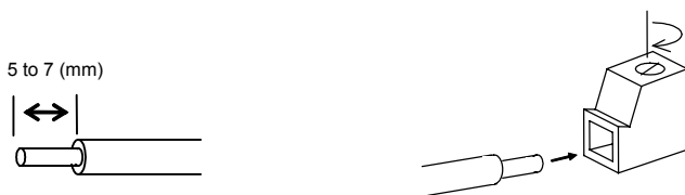
Figure 1.7 Stripping the Wire End Before Connection to Terminal Block
