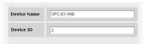
Figure 29: BACnet Device Identifiers
