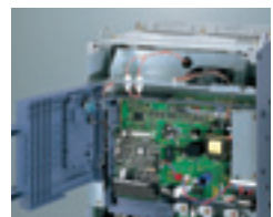
The inverter's mounting screws and power connector can be removed from the front.
