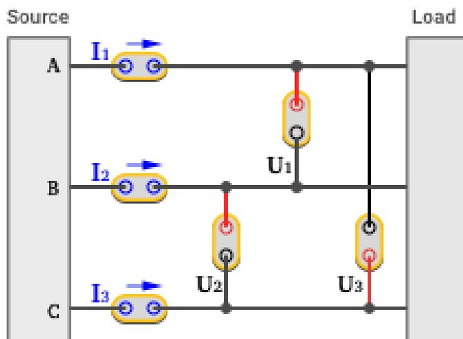
**Figure 10. 3P3W3M Wiring**
