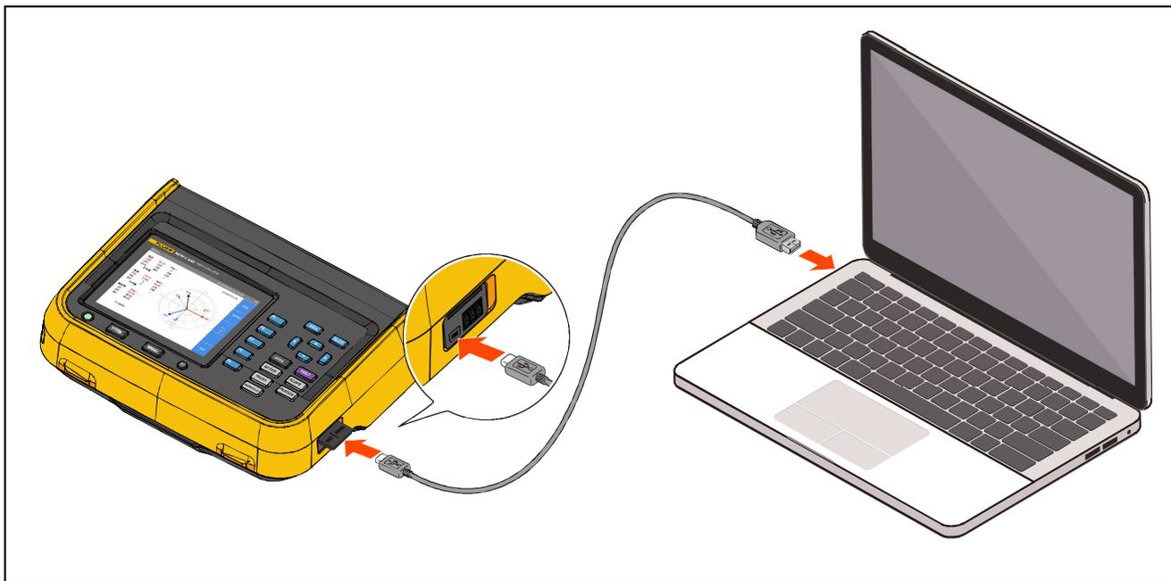
**Figure 22. Connect the Computer**
