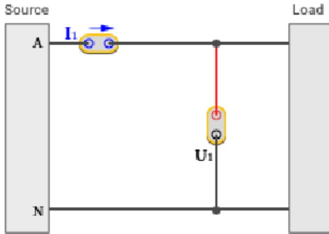
Figure 8. 1P2W1M Wiring
