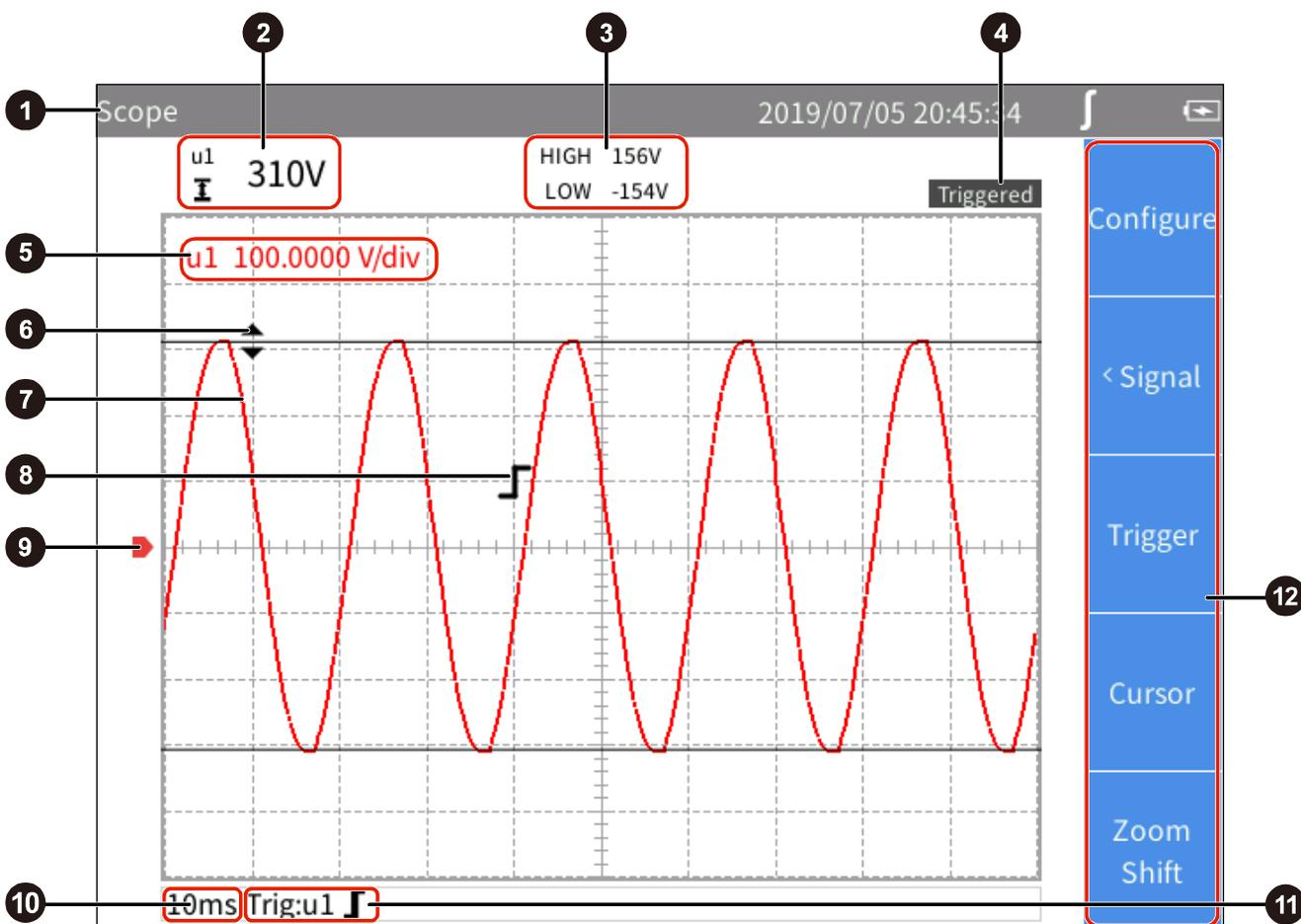
Figure 18. The Main Screen of Scope
