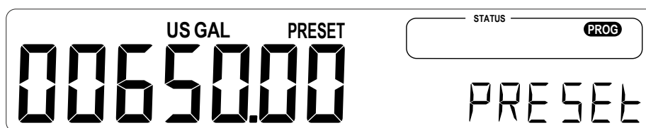
Fig. 4: Example display information during programming preset value
