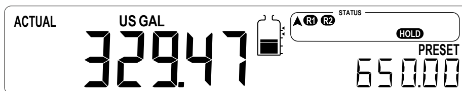
Fig. 6: Example display information when interrupted
