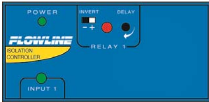
LC90 series faceplate: 1 sensor input, 1 relay output.
