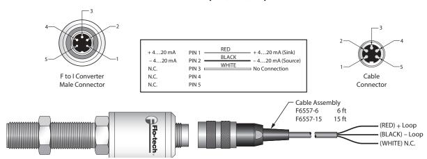
The 4...20 mA output can drive auxiliary devices (resistive loads) such as displays, recorders and computers, provided that the voltage supplied by the power supply is adequate. Devices must be wired in series with the F to I converter and power supply. The voltage drop across the load(s) and the 6V DC minimum needed to drive the F to I converter determine the minimum voltage required from the power supply.
