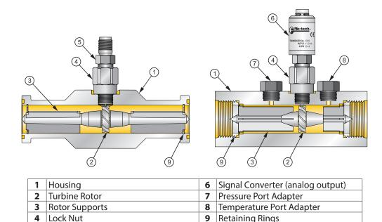
Turbine flow sensors measure the flow rate of hydraulic fluid and compatible liquids. As fluid flows through the sensor it turns the turbine rotor, and as the turbine blades pass the magnetic pickup a frequency signal is generated. This frequency signal is proportional to the flow rate and can be transmitted to Flo-tech's digital displays or converted to an analog output. Optional sensors allow measurement of pressure and temperature.
