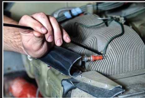
Inspecting cylinder in aircraft motor with VSA2-1M
