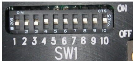
Figure 24. Ten-position DIP switch SW1.
