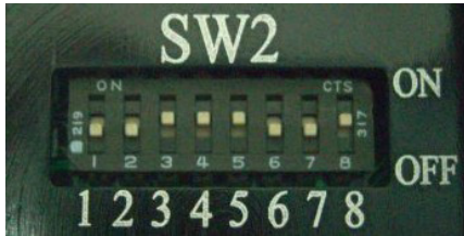
Figure 25. Eight-position DIP switch SW2
