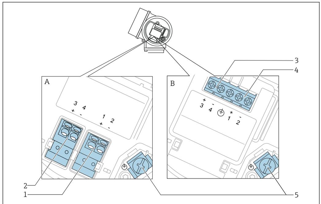
6 Terminal assignment 2-wire: 4-20 mA HART, 4-20 mA
