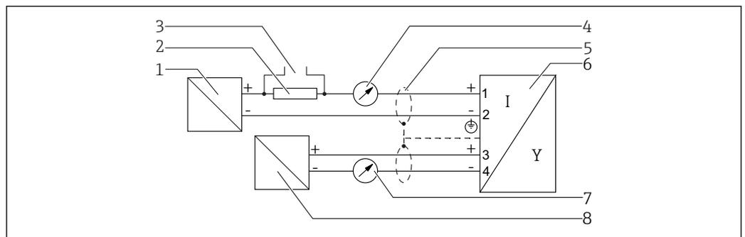
7 Block diagram 2-wire: 4-20 mA HART, 4-20 mA
