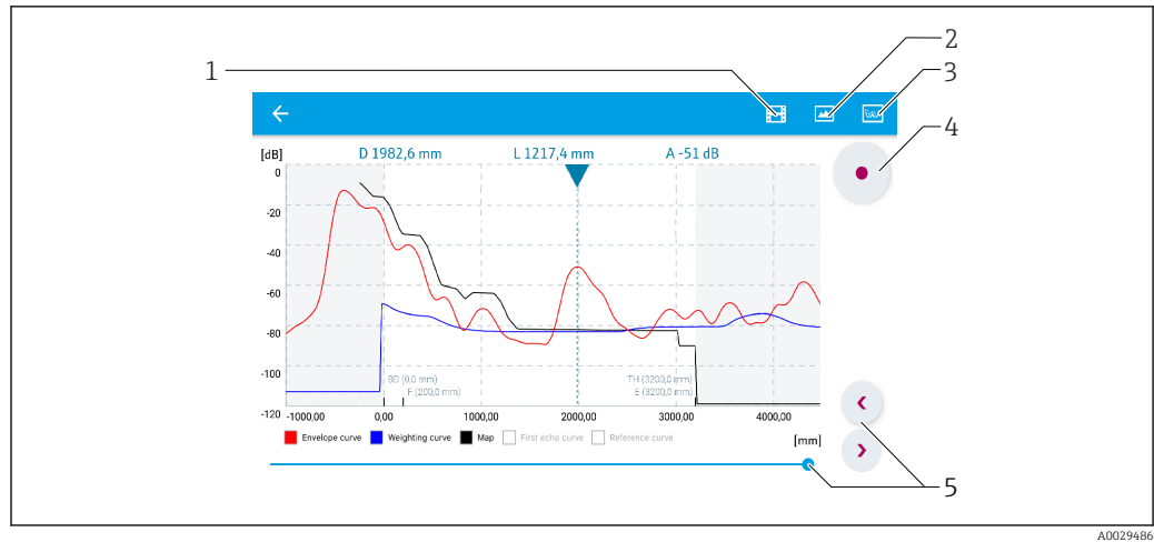
37 Envelope curve display (sample) in SmartBlue for Android
