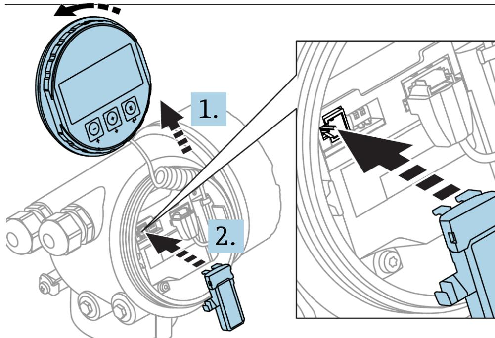
1. Open housing and remove the display
