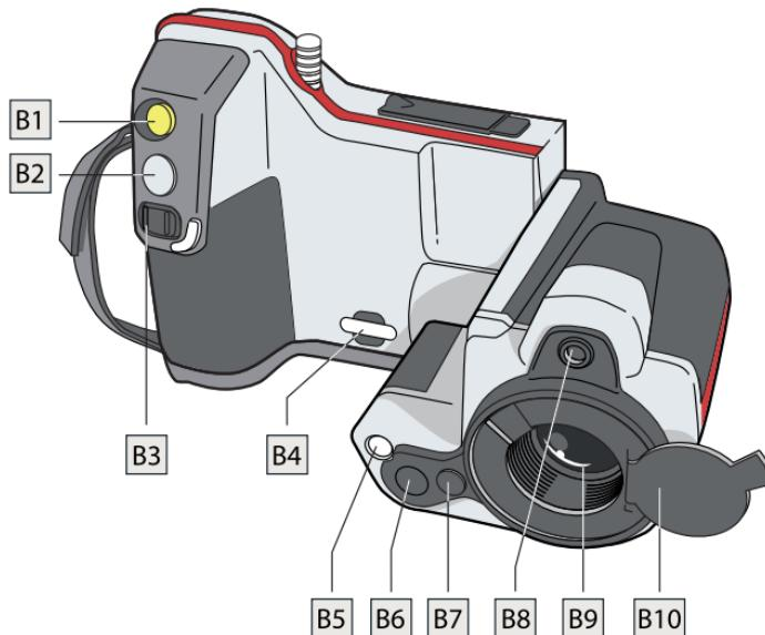
**B1.** Laser pointer button: Push to activate the laser pointer.
