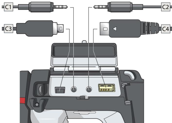
**C1.** To connect a headset to the camera to record and listen to voice annotations, use a headset cable and this socket.
