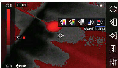
Figure 11.1 Above Alarm display
