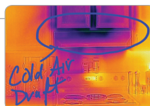
Sketch on IR/Visual -- Use Touchscreen to Draw Circles, Pointers, etc. on Stored Images
