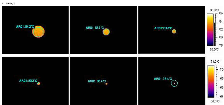
Figure 25.20 Temperature readings from a blackbody at +85°C (+185°F) at increasing distances (24° lens)
