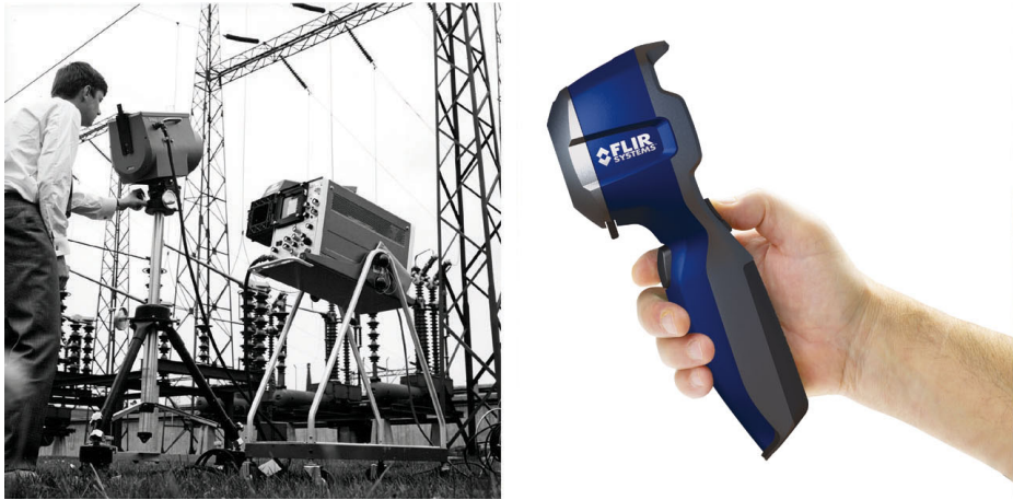
Figure 26.2 LEFT: Thermovision® Model 661 from 1969. The camera weighed approximately 25 kg (55 lb.), the oscilloscope 20 kg (44 lb.), and the tripod 15 kg (33 lb.). The operator also needed a 220 VAC generator set, and a 10 L (2.6 US gallon) jar with liquid nitrogen. To the left of the oscilloscope the Polaroid attachment (6 kg/13 lb.) can be seen. RIGHT: FLIR i7 from 2009. Weight: 0.34 kg (0.75 lb.), including the battery.
