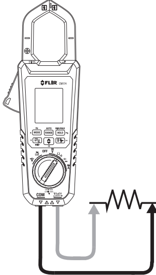
Figure 5.5 Resistance and Continuity Measurements
