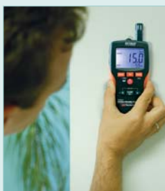
Measure moisture of wall material with non-invasive Pinless technology.
