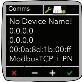
Figure 41 EPack 'Comms' screen display 'as-delivered' (Device Name = "", IP Configuration = Null).
