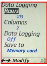
incorrectly the pressing Left or Right will move back or forwards between readings allowing a new reading to be taken and overwrite the existing value. When moving backwards and forwards, the previous reading at this location will not be shown.
