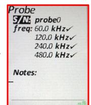
use that frequency. Pressing OK with no frequency highlighted will load in the probe file and use the first frequency in the list.
