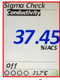
The Status Bar shows 4 Alarm LED representations, the temperature read by the probe, a MicroSD card icon and a Battery Meter or USB indicator.
