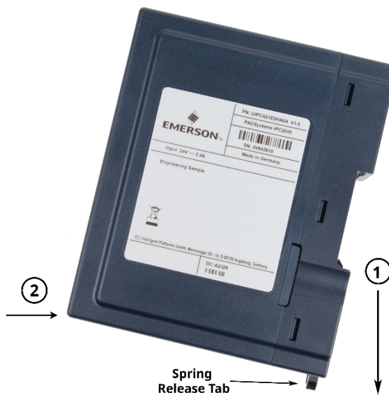
Figure 1: Attaching a DIN Rail to a IPC 2010
