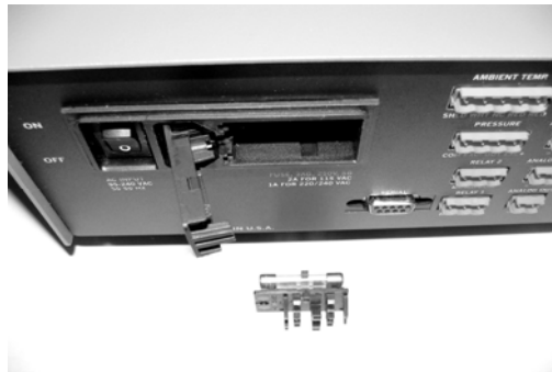
Figure 14-2b. Fuse Holder Removed
