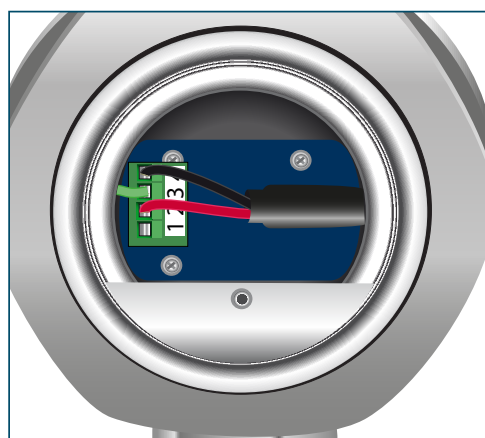
Figure 6 Terminal Block Connection
