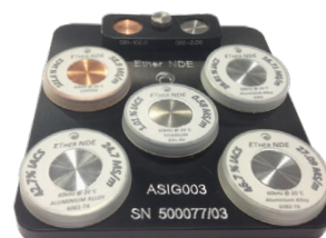
Conductivity Test Blocks in holder.
