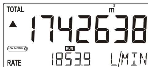
Fig. 4: Example of low-battery alarm.
