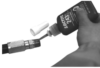
Figure 2: Apply thread sealant
