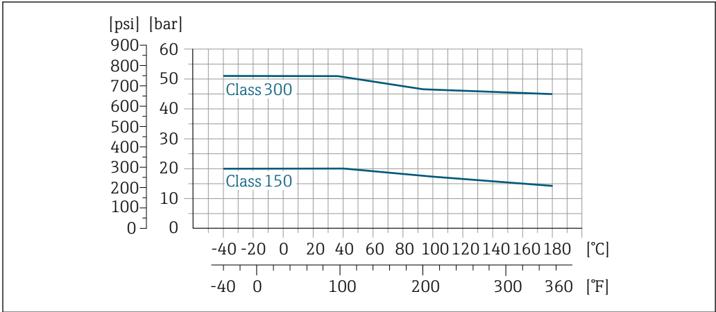
35 Process connection material: carbon steel, A105
