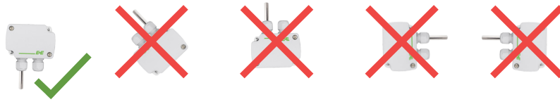
Fig. 5 Correct and incorrect mounting of the sensor
