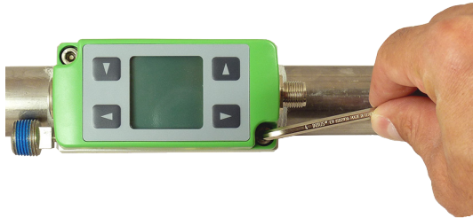
Fig. 23 Unscrew mounting screws
