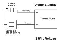
POWER SUPPLY ⁺\_\_\_ (+ Power) (Common) -T TRANSDUCER (+ Output METER OR OTHER DEVICE
