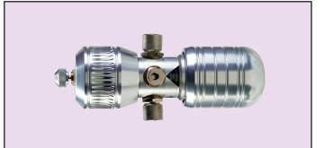
Model HP Hand Pump provides a dual source of pneumatic pressure and vacuum for verifying the calibration of pressure instrumentation. Pump can generate pressures up to 45 psig (3 bar) and vacuum to -27 in Hg (-910 mbar). The compact pump is designed for portability and single hand operation.
