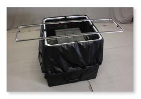
6. Assemble the required upper frame system that matches the adapter hood choice. Details for which pieces are needed for each hood size are on page 2. Starting with two pieces that fit together, loosen the knob on the first piece. Slide the second piece so the grooves fit around the knob on the first piece. Tighten the knob to hold in place. Continue until entire upper frame is assembled.
