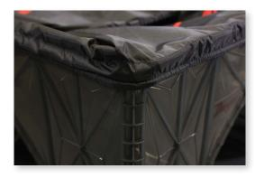
4. Fold the canvas hood inside out over the SAH, exposing the inner cord loop and place that cord loop inside the SAH unit. Pay special attention to the corners. Open the fabric hook and loop straps if they are closed.
