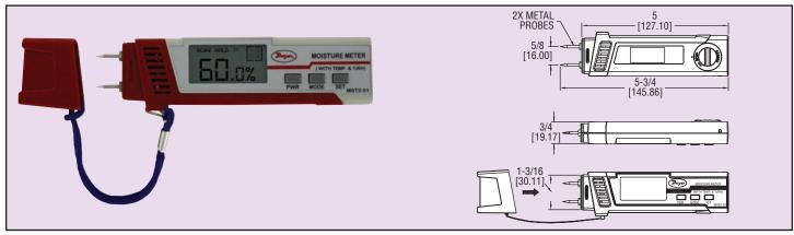
The Model MST2-01 Digital Moisture Meter is a high-accuracy instrument used for determining the moisture content in wood, gypsum, bamboo, paper and other various materials. This unit also has the ability to measure ambient temperature and relative humidity. The large digital LCD makes measurements easy to read, while the hold function makes them easy to record. The MST2-01 includes a protective cap, two replacement pins, and one battery.
