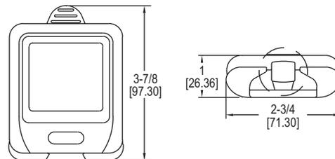
The **SERIES DW-WIFI** Wireless Wi-Fi Data Logger measures and records up to 1,000,000 temperature and/or humidity readings and shares the data with any PC or server on the same Wi-Fi network. If the Wi-Fi connection is lost, the sensor will continue to store any records until it can regain communication with the network. The downloadable Windows® based software allows users to set high/low alarms, sampling rate, and the temperature scale.
