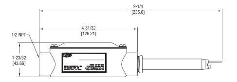
**The Series 641B Air Velocity Transmitter** uses a heated mass flow sensor technology. It has 4 user selectable ranges from 250 FPM to 2000 FPM with corresponding metric ranges of 1.25 MPS to 10 MPS. The 641B provides an isolated 4-20 mA output proportional to the velocity.
