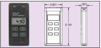
Series 490 Digital Manometers are versatile, hand-held, battery operated manometers available in several basic ranges for positive or positive differential pressure measurement and can tolerate most liquid media compatible with 316LSS. A memory function allows storage of up to 40 readings for later recall and a backlight provides auxiliary lighting for hard-to-see locations.
