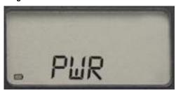
Push **ENTER** to see current time off setting. Select 30 or 10 values indicating minutes for power to automatically shut-off. By selecting 0, the auto shut-off is disengaged and the unit will only turn off manually by the ON/OFF/LIGHT button.
