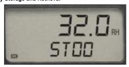
From the home screen, push **MEMORY/UP** to view all previously stored values. Cycle up or down through the stored data with the MEMORY/UP or STORE/DOWN buttons. From the home screen, press STORE/DOWN to store data points to memory. For both data storage and data memory retrieval, press **MENU** to return to the home screen.
