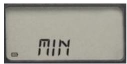
Push ENTER to see the minimum recorded reading. When viewing the minimum recorded reading, hold ENTER for 4 seconds to clear.
