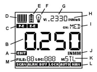
The **ZX-6 DL** uses a custom glass LCD backlit low temperature display for use in a variety of climate conditions. It contains graphic icons, as well as both 7 and 14 segment display areas. Let's take a closer look and what all these things are telling us:
