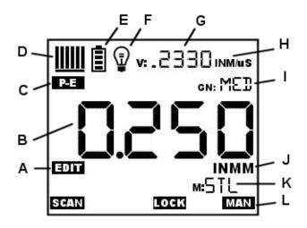
The *R9* uses a custom glass LCD backlit low temperature display for use in a variety of climate conditions. It contains graphic icons, as well as both 7 and 14 segment display areas. Let's take a closer look and what all these things are telling us:
