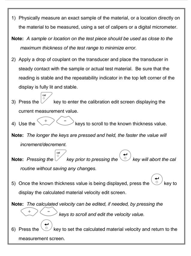
CHECK YOUR CALIBRATION! Place the transducer back on the calibration
