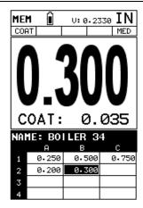
1) Press the MENU key once to activate the menu items tab. Press the MENU key multiple times to tab right and the ESC key multiple times to tab left until the DATA menu is highlighted and displaying the submenu items.
