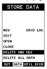
2) Use the **UP** and **DOWN** arrow keys to scroll through the sub menu items until **DELETE ONE FILE** is highlighted.
