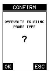
6) Press the **OK** key to overwrite the existing probe type, or **ESC** to cancel.
