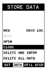
2) Use the **UP** and **DOWN** arrow keys to scroll through the sub menu items until **CLOSE** is highlighted.
