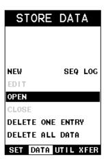
2) Use the **UP** and **DOWN** arrow keys to scroll through the sub menu items until **OPEN** is highlighted.
