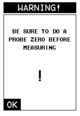
**Note:** The probe zero disk (battery cap) is located on the top end cap of the gauge. The warning screen will be displayed following the selection and overwrite of a new transducer.
