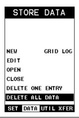
2) Use the **UP** and **DOWN** arrow keys to scroll through the sub menu items until **DELETE ALL DATA** is highlighted.
