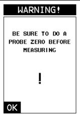
7) The zero probe warning screen will be displayed. Press the **OK** key, followed by pressing the **MEAS** key to return to the main measurement screen and proceed to the probe zero section that follows.
