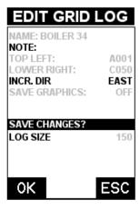
10)Press the **UP** or **DOWN** arrow key to highlight **SAVE CHANGES**, and the **OK** key to activate the confirmation screen.
