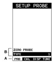
1) Press the MENU key once to activate the menu items tab. Press the MENU key multiple times to tab right, and the ESC key multiple times to tab left until the desired tab group is highlighted and displaying the submenu items. The tab groups are illustrated above (A).
