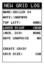
Use the UP and DOWN arrow keys to scroll through the setup list until LOWER RIGHT is highlighted. 2) Press the ENTER key to activate the Coordinate Edit Box.
