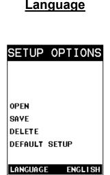
Press the MENU key once to activate the menu items tab. Press the MENU key multiple times to tab right and the ESC key multiple times to tab left until the SETUP menu is highlighted and displaying the submenu items.
