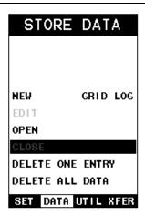
3) Press the **ENTER** key to close the active file. **Note:** Following the key press, the **CLOSE** text will be grayed out indicating the file has been close and is no longer active.
