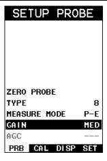
Press the MENU key once to activate the menu items tab. Press the MENU key multiple times to tab right, and the ESC key multiple times to tab left, until the PRB menu is highlighted and displaying the submenu items.
