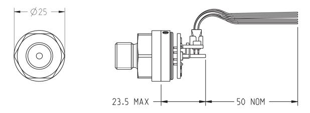
GAUGE SENSOR WITH PB PRESSURE CONNECTOR SHOWN
