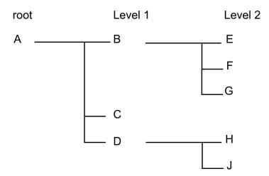
In the command tree the command A is the root command. A tree pointer is used to decode the SCPI commands. At power-up the pointer goes to the root command.
