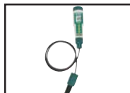
Extension cable attached to meter
