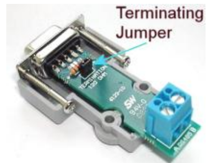
Fig 3-19 RS485 120 Ohm Jumper
