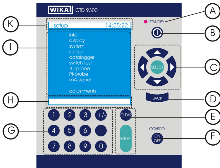
Fig. 2: User Interface of a CTD9300
