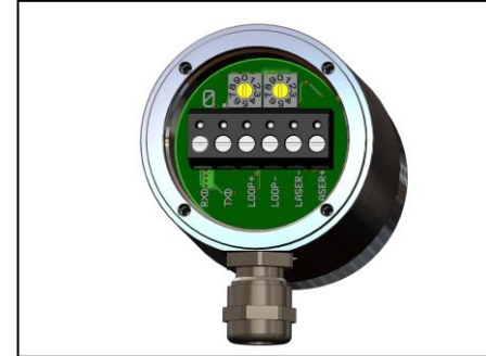
Sensor back side with terminal block
