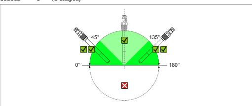
*Installation angle for Memosens COS81D-\*\*\*\*U\*\*\* (u-shaped spot cap)* € 4
