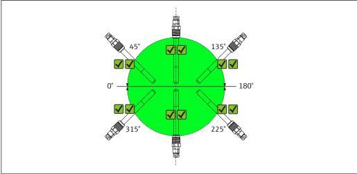
*Installation angle for Memosens COS81D-\*\*\*\*C\*\*\* (c-shaped spot cap) The sensor can be installed at any installation angle (0 to 360°).*
