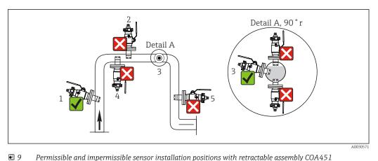
Permissible and impermissible sensor installation positions with retractable assembly COA451
