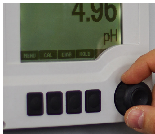
34 Operation via external, optional display
