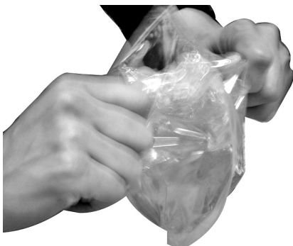
Figure 5: Knead the bag to mix the resin
