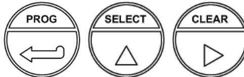
Fig. 2: Control panel, optical keys
